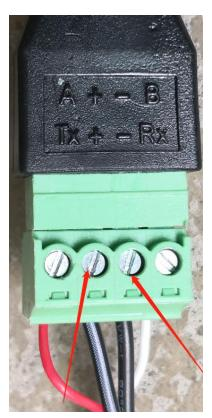
The power plug is connected to a 230V power supply. The black and white line of the power cord is connected to the + of the connection line, and the black line is connected to the-of the connection line. If the connection is reversed, the module cannot supply power.
